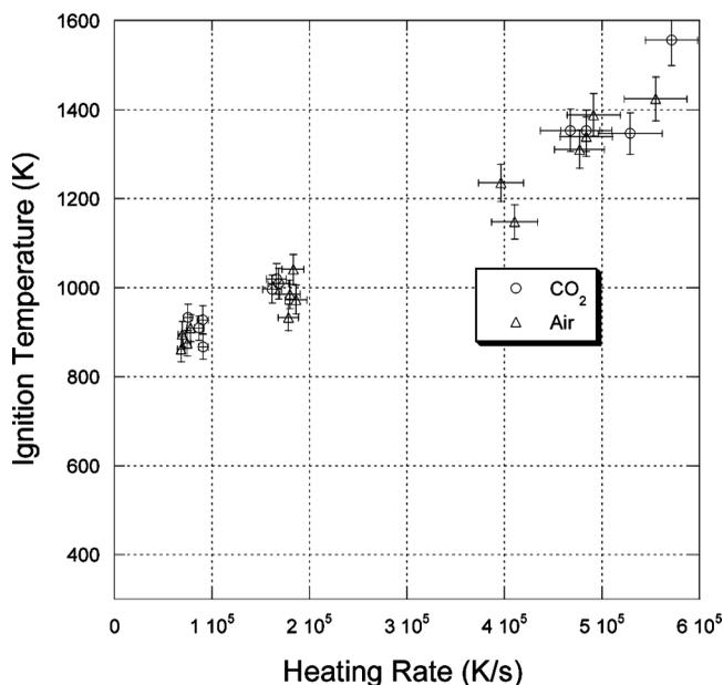
Figure 11 Ignition temperature of AlH<sub>3</sub> in air and CO<sub>2</sub> as a function of heating rate.
