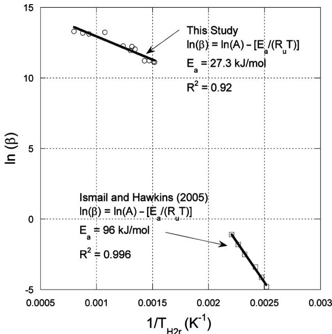
Figure 9 Arrhenius plot of  $AlH_3$  hydrogen release.
