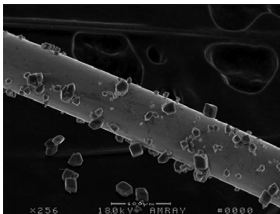
Figure 2 SEM image of  $\text{AlH}_3$  on platinum filament.
