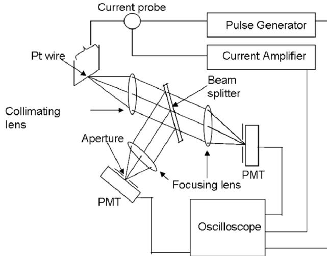
Figure 3 Schematic diagram of T-Jump optical emission system.
