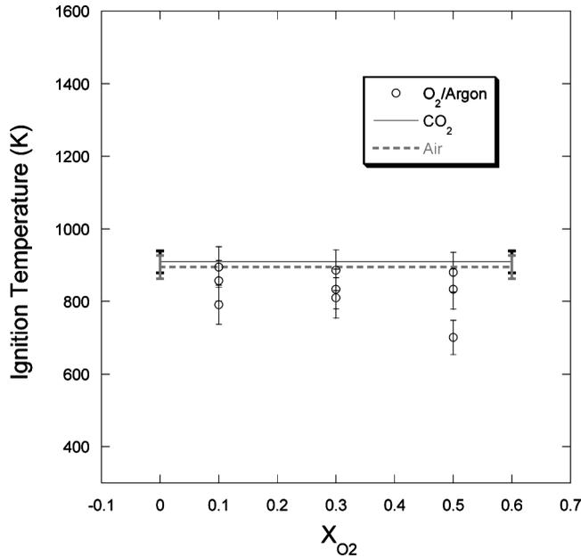
**Figure 13** Ignition temperature of AlH<sub>3</sub> in Ar/O<sub>2</sub> Mixtures for a heating rate of  $\sim 7 \times 10^4$  K/s.
