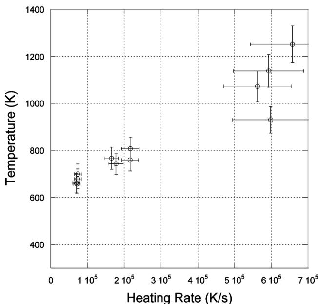
**Figure 8** Hydrogen release temperature from AlH<sub>3</sub> as a function of heating rate.
