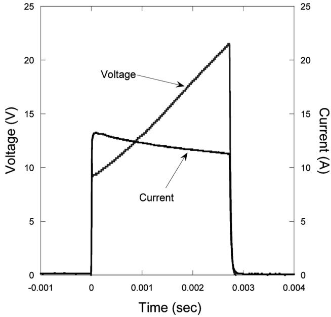
**Figure 4** Typical voltage and current trace from 76  $\mu\text{m}$  Pt wire for heating rate of  $\sim 5 \times 10^5$  K/s.
