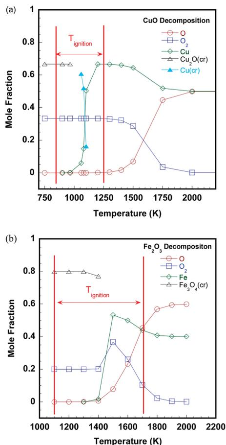
**Figure 7.** Results of thermal equilibrium calculation using CEA code for (a) CuO decomposition and (b) Fe<sub>2</sub>O<sub>3</sub> decomposition.  $T_{\text{ignition}}$  is ignition temperature of nanocomposite reactions measured from T-Jump/TOFMS.
