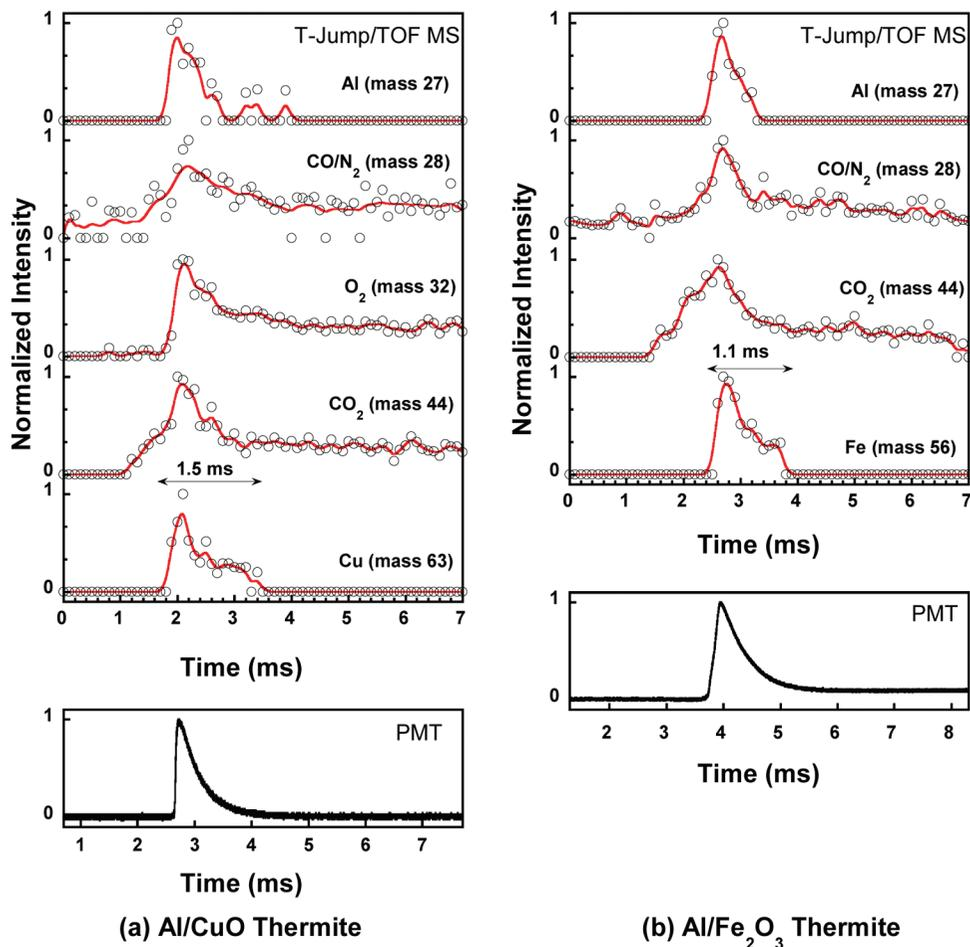
**Figure 8.** Normalized peak intensities as function of reaction time for reaction species observed in (a) Al/CuO and (b) Al/Fe<sub>2</sub>O<sub>3</sub> reactions; the bottom plots are optical signal measured from separated experiments.
