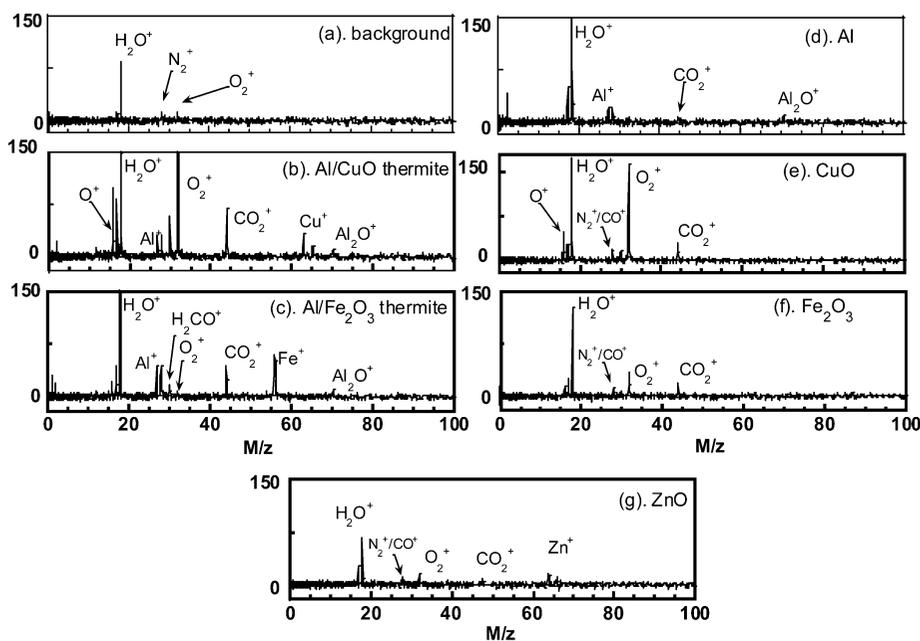
**Figure 5.** Detailed views of selected mass spectra obtained from T-Jump experiments. (a) Background, (b) Al/CuO mixture, (c) Al/Fe<sub>2</sub>O<sub>3</sub> mixture, (d) Al particles, (e) CuO particles, (f) Fe<sub>2</sub>O<sub>3</sub> particles, (g) ZnO particles.
