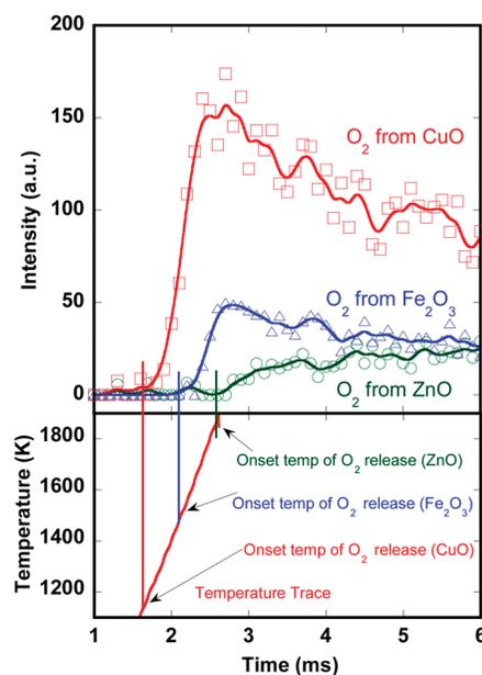
**Figure 6.** Temporal profile of oxygen peak intensity from heating of CuO, Fe<sub>2</sub>O<sub>3</sub>, and ZnO nanoparticles.
