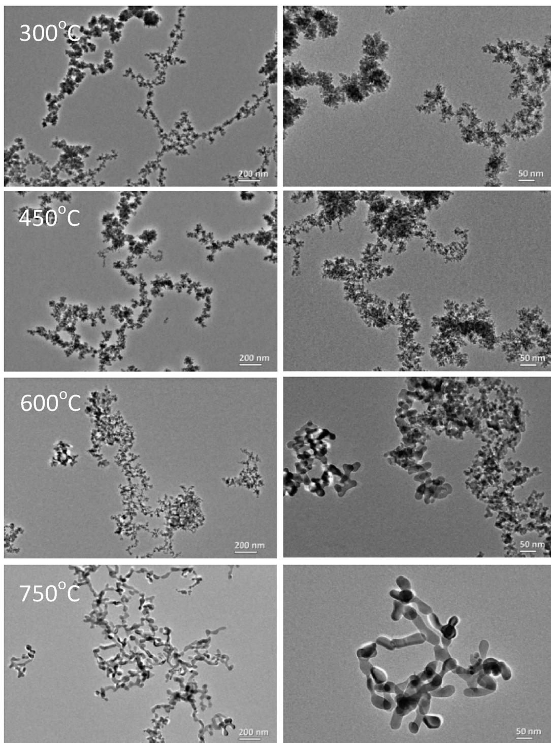
**Figure 8.** TEM images of Fe NPs at different reactor temperatures.
