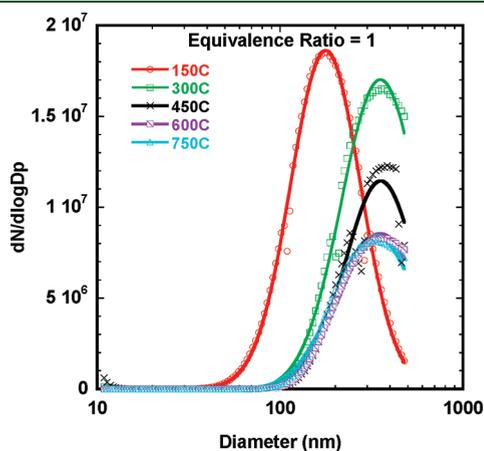
Figure 9. Particle size distributions of Fe NPs at different temperatures.
