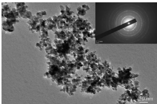
Figure 2. TEM image of Fe aggregates.
