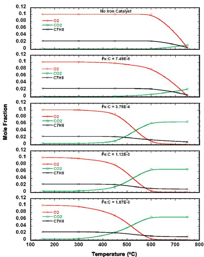
Figure 7. Mole fraction of toluene, CO<sub>2</sub>, and O<sub>2</sub> for experiments of different Fe catalyst loading at an equivalence of 2.3.
