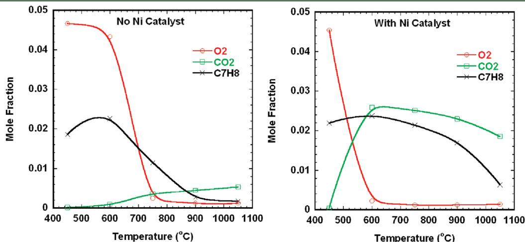
Figure 10. Toluene ignition catalyzed by Ni NPs.
