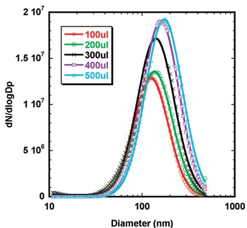
Figure 3. Particle size distribution of iron NP aggregates generated by iron carbonyl decomposition at 150 °C with different iron precursor concentrations.
