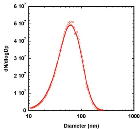
Figure 4. Particle size distribution of Ni NPs generated by nickel tetracarbonyl decomposition at 450 °C.
