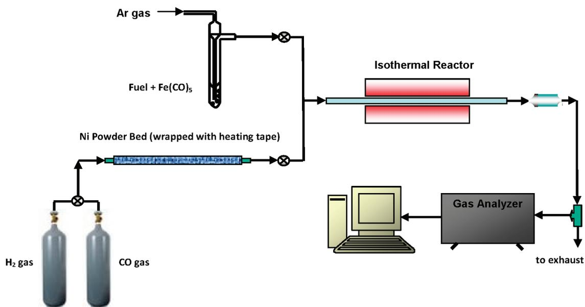
Figure 1. Schematic of the experimental setup for liquid fuel ignition.
