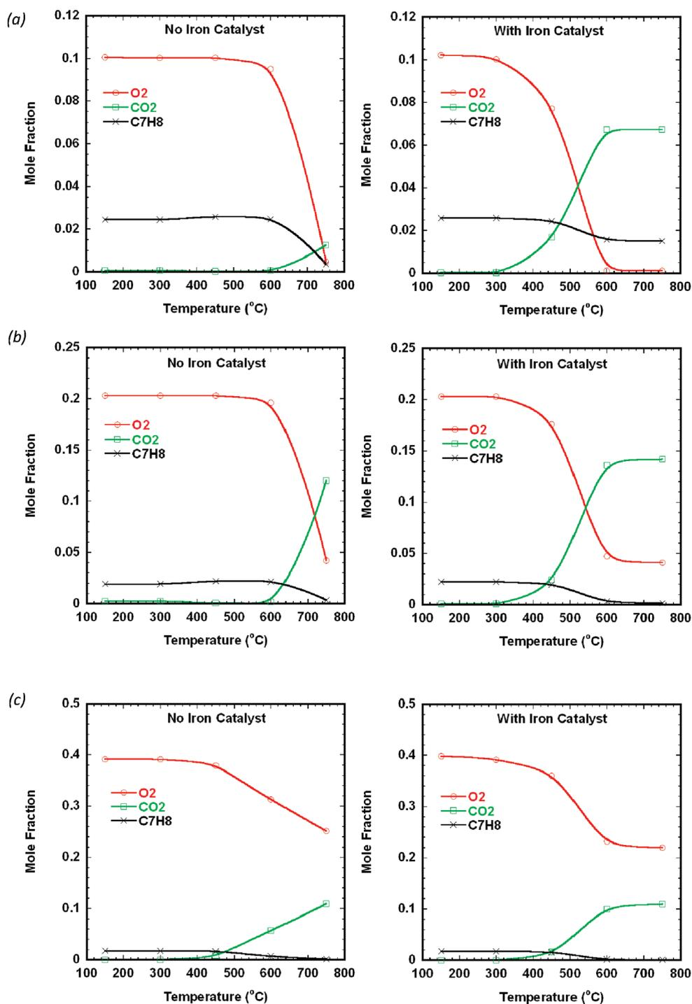
**Figure 6.** Mole fraction of fuel (toluene), oxidizer (O<sub>2</sub>), and products (CO<sub>2</sub>) for a fuel/oxidizer equivalence ratio of (a) 2.3, (b) 1.0, and (c) 0.4.
