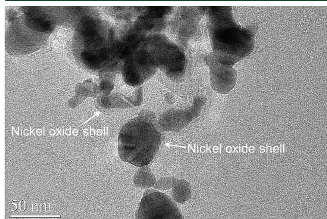
Figure 11. TEM image of Ni catalyst particles reacted at 750 °C.
