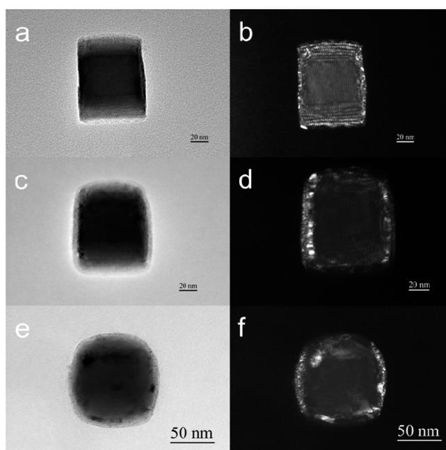
**Figure 4.** (a and b) Bright and dark field images of a side surface deposited NC before heating; (c and d) bright and dark field images taken after heating the NC at 300°C for ~5 minutes; (e and f) bright and dark field images taken after heating the NC at 325°C for ~6 minutes, the NC transforms into a spherical shape.
