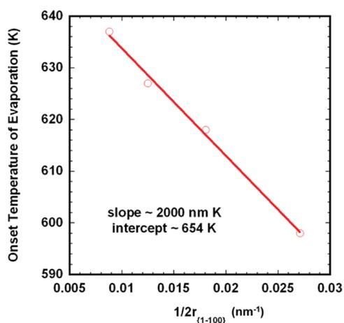
Figure 6. Onset temperature of evaporation vs  $1/2r_{\{1\bar{1}00\}}$ .
