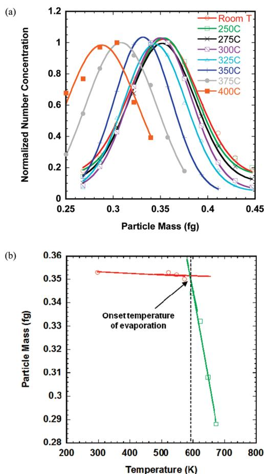
**Figure 5.** (a) Normalized particle mass distributions for the initial mobility NC size of 50 nm at different evaporation temperatures. (b) Particle mass vs temperature for the initial NC size of 50 nm. The intersection of two straight lines is the onset temperature of evaporation.
