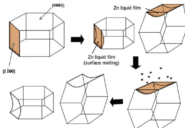
**Figure 3.** Evaporation mechanism of free Zn NC.
