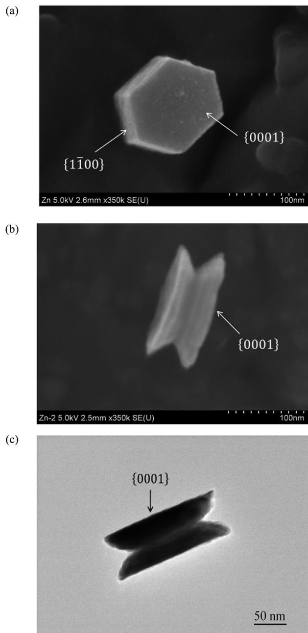
**Figure 2.** Images of aerosol grown hexagonal-prism-shaped Zn NCs: (a) SEM image of a Zn NC before evaporation, (b) SEM image of a partially evaporated Zn NC, and (c) TEM image of partially evaporated Zn NC.
