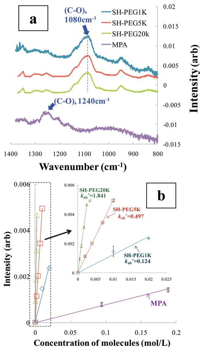
**Figure 2.** Quantitative analysis of free ligand concentration in DI water using ATR-FTIR. (a) IR spectra of unbound ligands in water. From top to bottom: SH-PEG1K, SH-PEG5K, SH-PEG20K, and MPA. The ligand mass fraction is 2% for all spectra. (b)  $I_{ab}$  vs  $C_m$  for SH-PEG1K (diamonds), SH-PEG5K (squares), SH-PEG20K (triangles), and MPA (crosses). Data are fit using linear regression with a slope  $k_{ab}^*$ .
