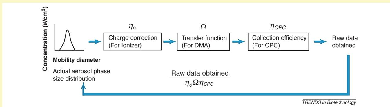
**Figure I.** Data processing in the ES–DMA. The raw counts are corrected for charge correction, transfer function of the DMA and collection efficiency (if a CPC is used for counting).
