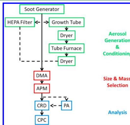
**Figure 1.** Schematic diagram of the system used to generate soot aerosol, tune its morphology, size, and mass select particles and measure absorption or extinction and number density. HEPA filter was included to collect background optical measurements. Dashed lines indicate optional flows.
