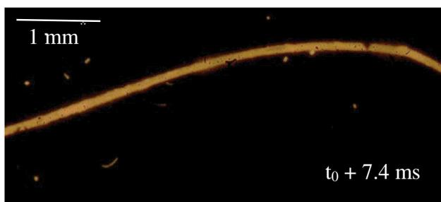
**Figure 6.** T-jump ignition of sample 4 at 0.101 MPa in air.
