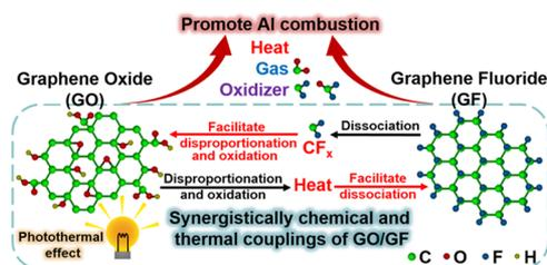
**Figure 1.** Proposed mechanism for GO/GF chemical and thermal couplings. Schematics of the synergistically thermal and chemical coupling between GF and GO and its effects for enhancing the energetic performance of Al (green, C atoms; red, O atoms; blue, F atoms; yellow, H atoms).
