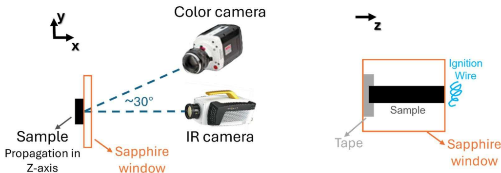
FIG. 1. Experiment setup of the combustion tests. (Note: the combustion chamber was not shown and the objects were not drawn to scale.)
