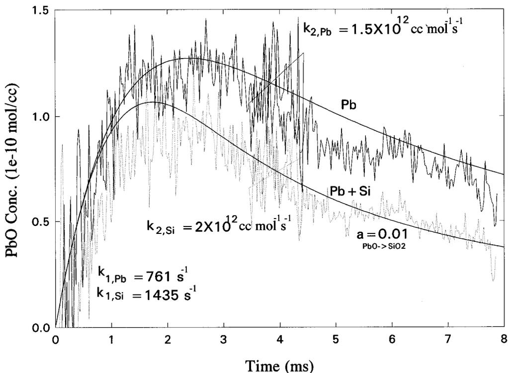
FIGURE 4. Centerline profile of PbO(g) concentration as a function of time from the flame front for a lead only feed rate (case 1) and lead-silicon co-feed (case 2).
