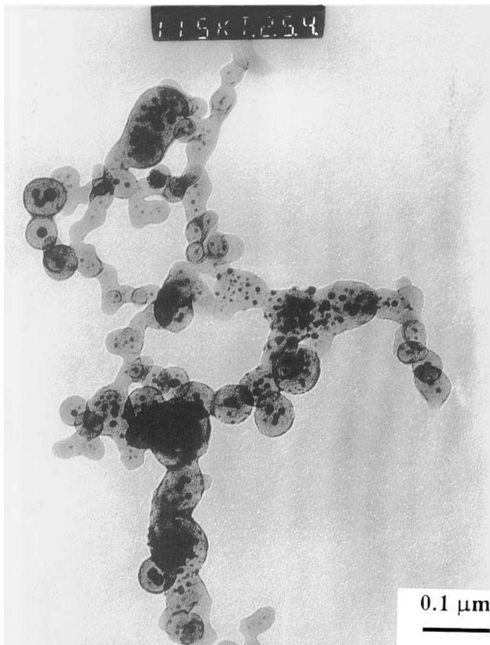
FIGURE 7. Transmission electron micrograph of the resultant lead-silica composite particles formed. The dark regions are the lead silicate compound dispersed in a silica matrix.
