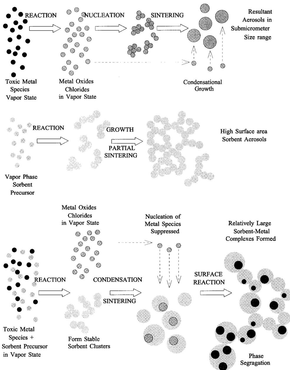
FIGURE 6. Mechanistic representation of the lead-silicon reaction system.
