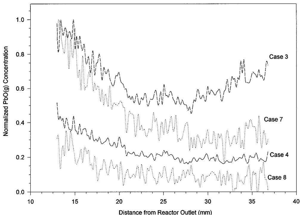
FIGURE 5. Centerline profile of normalized (by concentration at exit of furnace for a lead only feed) PbO(g) concentration for the furnace experiments as a function of distance from the exit of the reactor for cases 3, 4, 7, and 8.
