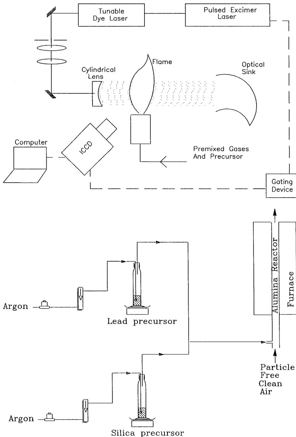
FIGURE 1. Schematic diagram of experimental system. (a) Premixed flame system; (b) furnace reactor system.
