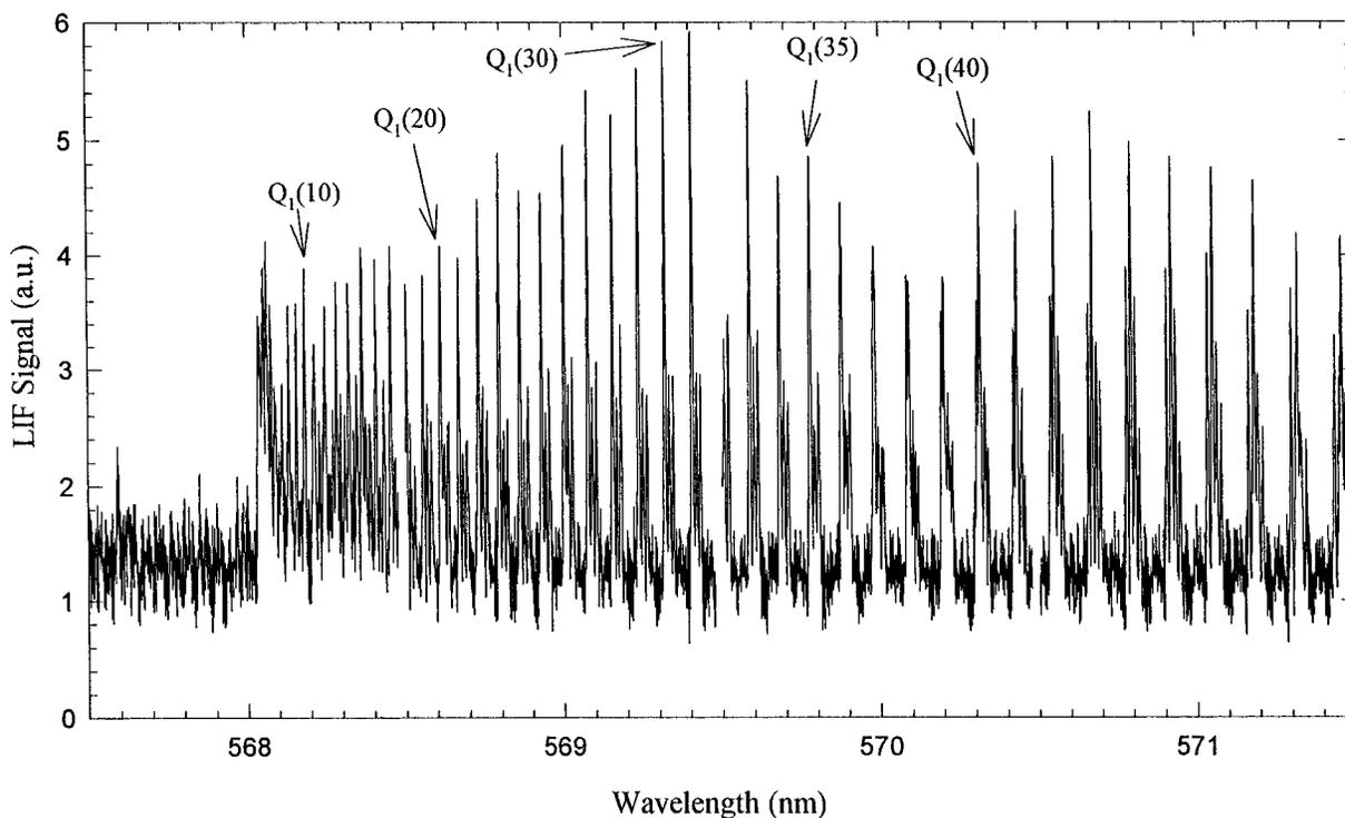
FIGURE 2. Laser excitation spectrum of PbO between 567.5 and 571.5 nm established with a resolution of 0.001 nm. Also shown are rotational states for a few lines.
