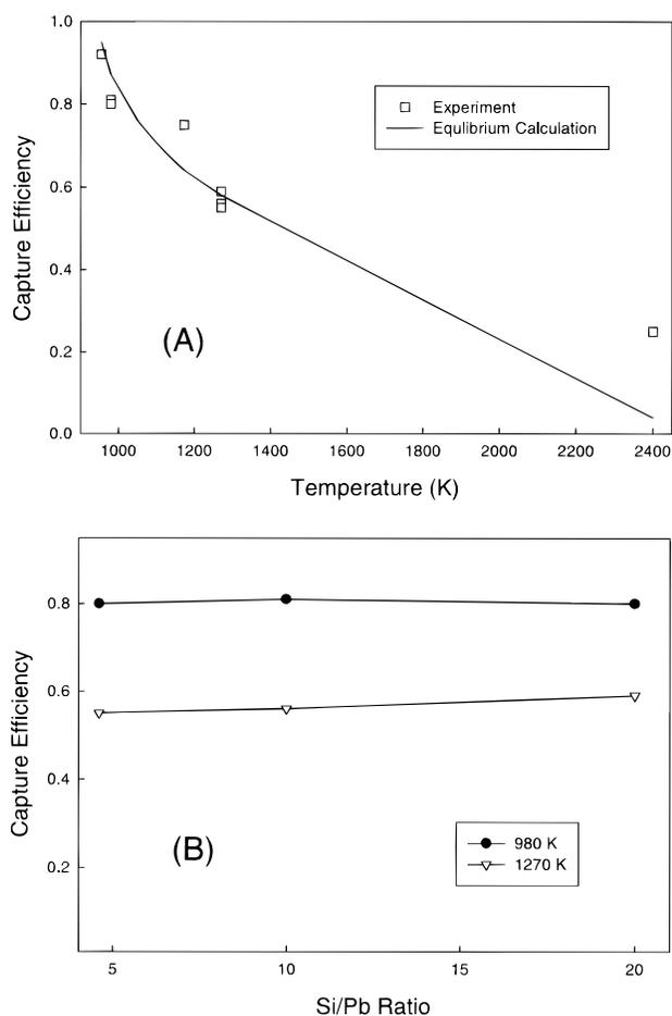
FIGURE 8. (A) Capture efficiency of lead species as a function of temperature. Symbols represent the experimental data, and the line represents the results of an equilibrium calculation. (B) Capture efficiency of the lead species as a function of the Si/Pb ratio at two temperatures. The symbols represent the experimental data, and the lines represent the results of equilibrium computations.
