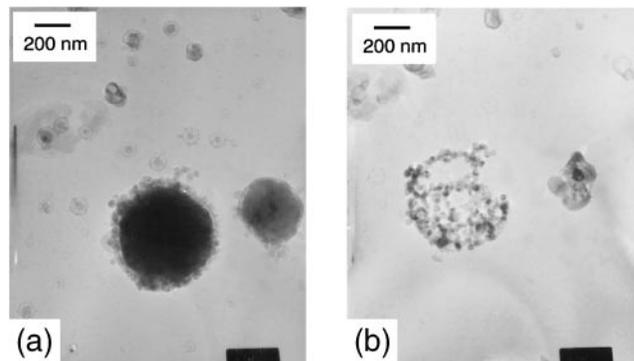
FIG. 11. Transmission electron microscope images of silicon particles formed at 1023 K: (a) salt-coated particles and (b) the same particles with the salt coating removed.
