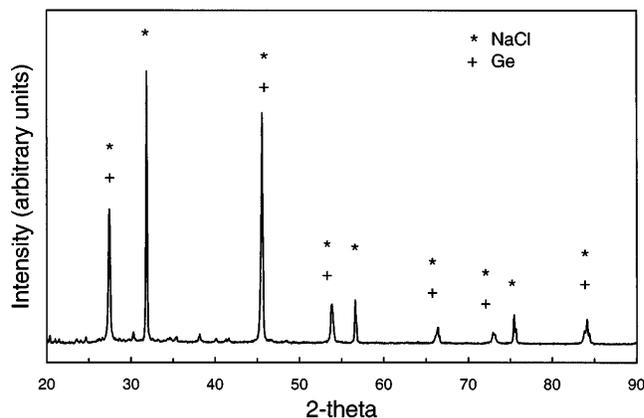
FIG. 8. X-ray diffraction pattern of salt-encapsulated germanium particles, showing the absence of any oxides.
