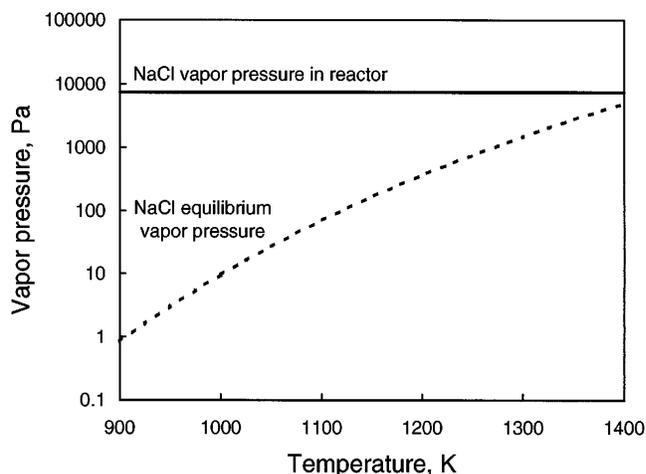
FIG. 5. Equilibrium vapor pressure of salt as a function of temperature. Solid line shows vapor pressure of salt in furnace region assuming complete reaction between precursor and salt.
