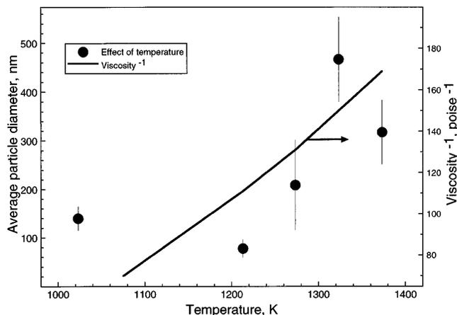
FIG. 13. Variation of particle size with furnace temperature for germanium. Vertical bar is equal to  $\pm$  the standard deviation of the particle size measurements.
