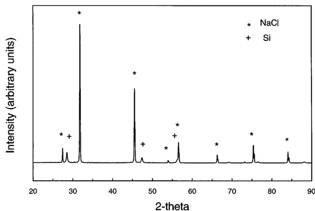
FIG. 7. X-ray diffraction pattern of salt-encapsulated silicon particles. The two phases present are metallic silicon and salt, indicating that the particles are not oxidized.
