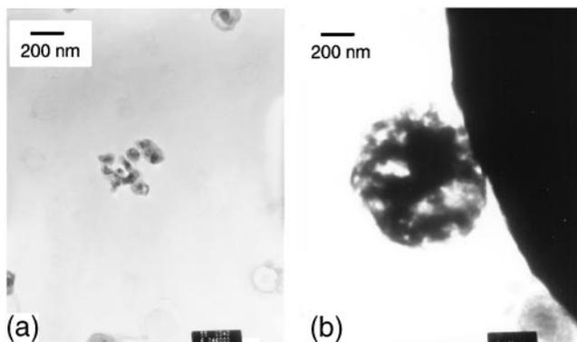
FIG. 10. Transmission electron microscope images of particles formed at 1213 K: (a) particles of silicon with the salt coating removed and (b) particles of germanium with the salt coating removed.
