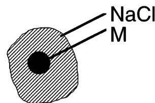
FIG. 1. Desired morphology for products of the salt-encapsulation process.
