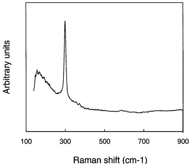
FIG. 9. Raman spectrum of salt-encapsulated germanium particles. Peak at  $\sim 300 \text{ cm}^{-1}$  corresponds to the first-order transverse optical phonon mode of germanium.
