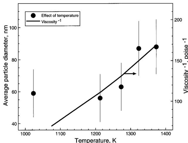
FIG. 12. Variation of particle size with furnace temperature for silicon. Vertical bar is equal to  $\pm$  the standard deviation of the particle size measurements.
