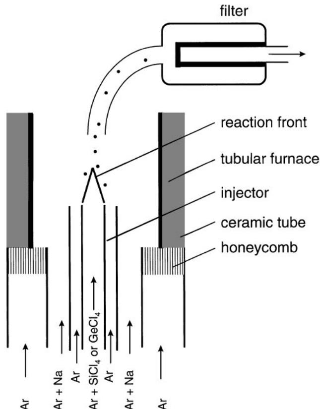
FIG. 4. A schematic of the cylindrical co-flow sodium reactor.
