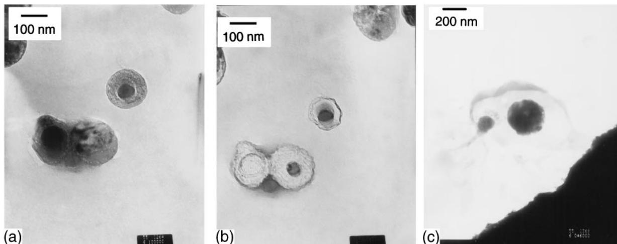
FIG. 6. Transmission electron microscope images of silicon and germanium particles formed at a furnace temperature of 1373 K: (a) coated silicon particles, (b) the same silicon particles shown in (a) with the salt coating removed, and (c) particles of germanium with the coating removed.
