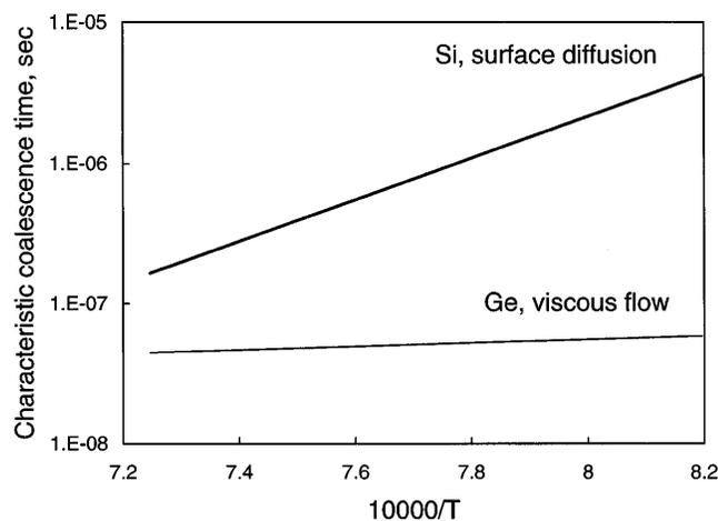
FIG. 3. Characteristic coalescence times calculated for silicon and germanium using Eqs. (3) and (5), respectively.
