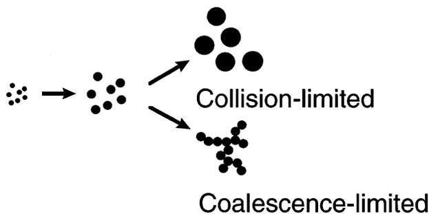
FIG. 2. Schematic showing unagglomerated particles resulting from collision-limited growth and agglomerates resulting from coalescence-limited aerosol growth.
