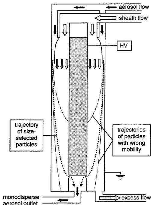
**Figure 3.** Schematic view of the DMAs used in this work. Particles with mobilities outside the desired range either hit and stick to the center rod electrode or go past the sampling slot and are carried away in the excess flow.
