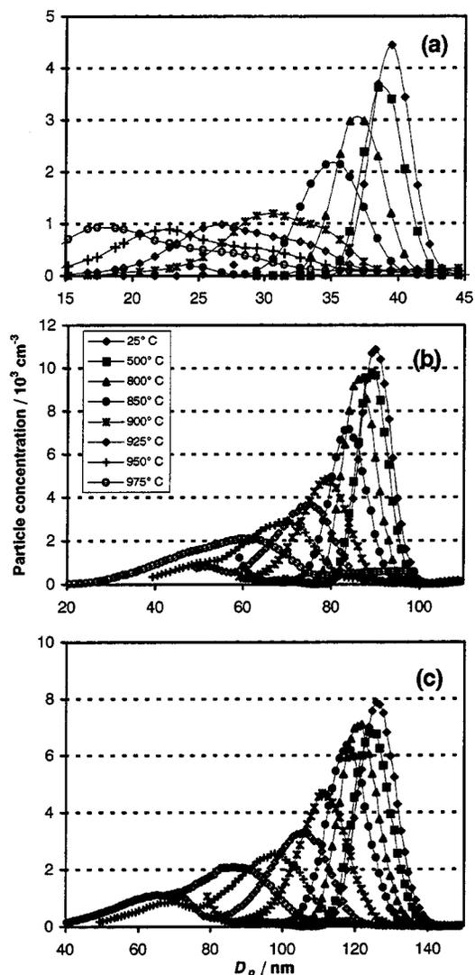
**Figure 8.** TDMA soot oxidation results in air for furnace settings of 25–975 °C (see legend). Results from higher furnace settings are omitted for clarity: (a) 40 nm initial particle size; (b) 93 nm initial particle size; (c) 130 nm initial particle size.
