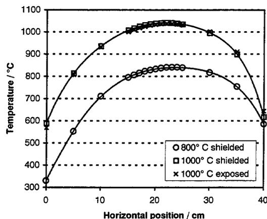
**Figure 4.** Temperature profiles within the quartz flow tube for furnace settings of 800 or 1000 °C. The data represented by open circles and squares were measured using a thermocouple shielded with a coil of iron wire, while the crosses show measurements made with an exposed thermocouple. The heated section of the furnace runs from a horizontal position of 5–35 cm.
