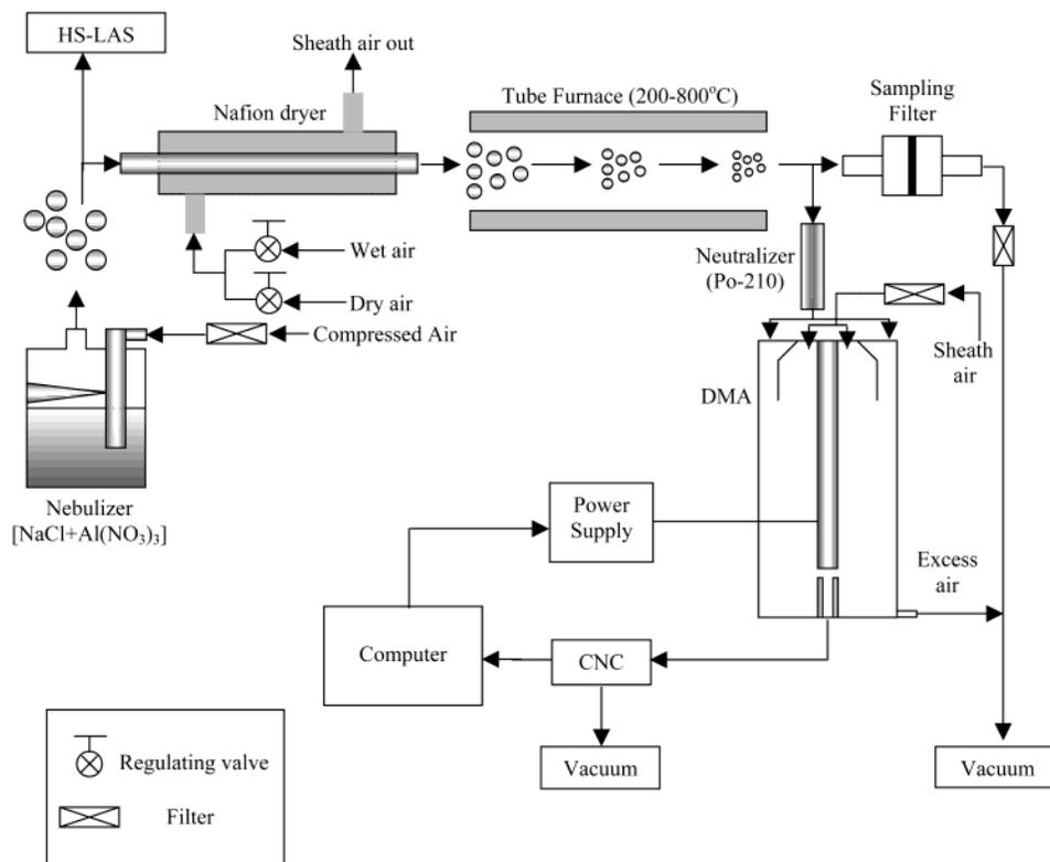
**Figure 1.** Schematic diagram of the experimental setup for synthesis and characterization of nanoporous particles. (DMA: differential mobility analyzer, CNC: condensation nuclei counter, HS-LAS: high-sensitivity laser aerosol spectrometer).
