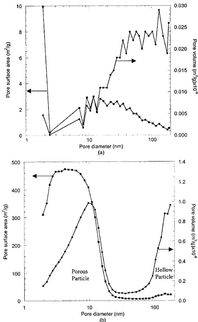
**Figure 7.** Pore surface area and volume distribution: (a) before and (b) after salt removal ( $\text{Al}(\text{NO}_3)_3\text{:NaCl} = 1\text{:}1$  at 1 wt % solution, synthesis temperature 550 °C, relative humidity = 30%).
