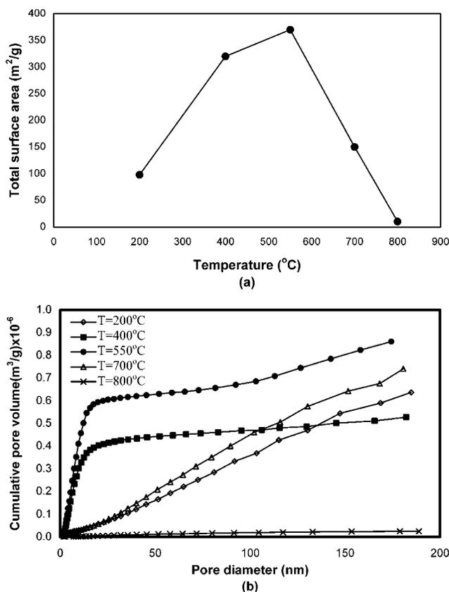
**Figure 8.** (a) Total pore surface area and (b) pore volume distribution for varying furnace temperatures ( $\text{Al}(\text{NO}_3)_3\text{:NaCl} = 1\text{:}1$  at 1 wt % solution, relative humidity = 30%, post NaCl removal).
