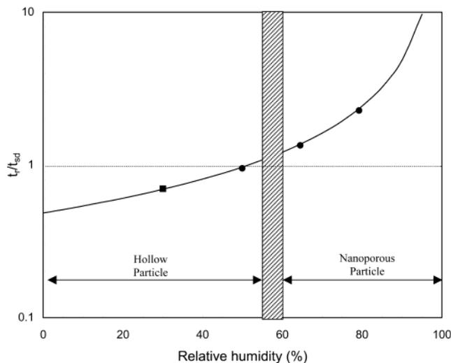
**Figure 13.** Ratio of characteristic time for droplet shrinkage to solute diffusion, as a function of relative humidity ( $t_i$  = characteristic time for droplet shrinkage,  $t_{sd}$  = characteristic time for solute diffusion; ● = Nafion membrane dryer, ■ = silica gel diffusion dryer).
