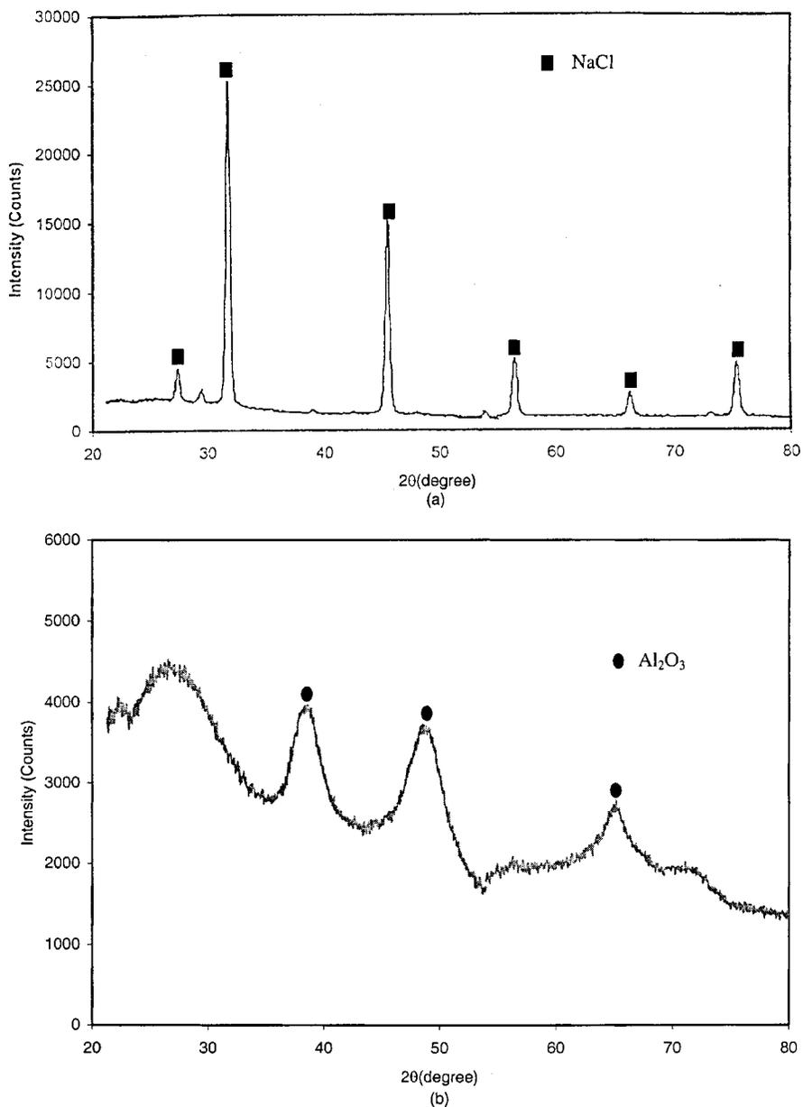
**Figure 5.** X-ray diffraction patterns of spray-pyrolyzed (a) Al<sub>2</sub>O<sub>3</sub> and NaCl ( $T = 550$  °C, before the washing process) and (b) Al<sub>2</sub>O<sub>3</sub> particles ( $T = 550$  °C, after the washing process).
