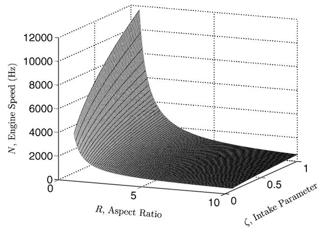
Fig. 5. The engine speed dependence upon the aspect ratio and intake conditions for a 10 W engine,  $r = 25$ .  $\zeta = 1.0$  corresponds to  $P_i = 1$  atm,  $T_i = 300$  K, and  $\Phi = 1.0$ .
