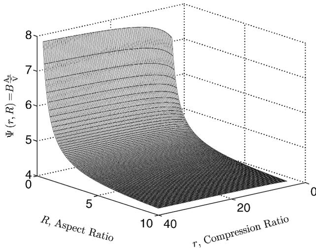
Fig. 8. Non-dimensional surface-area-to-volume ratio function, Eq. (27).
