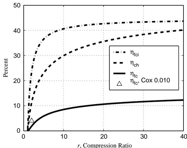
Fig. 3. The dependence of the charging and fuel conversion and efficiencies upon the compression ratio and comparison to the Cox 0.010 Glow-Ignition Model Airplane engine (Yang, 2000). Note that  $\eta_{fc} = \eta_{fc,i} \eta_{ch} \eta_m$  and that  $\eta_m = 0.70$ .
