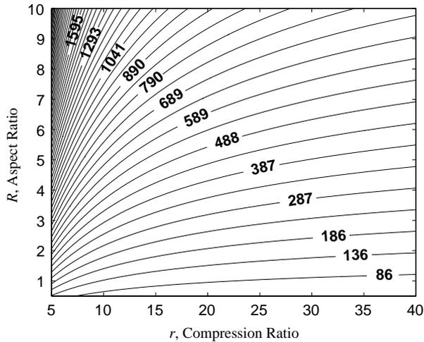
Fig. 6. Total cylinder volume,  $V_t$  ( $\text{mm}^3$ ) required to deliver 10 W when operating with a mixture of propane and air,  $\Phi = 0.5$ ,  $T_i = 500$  K and  $P_i = 1$  atm ( $\zeta = 0.3$ ).
