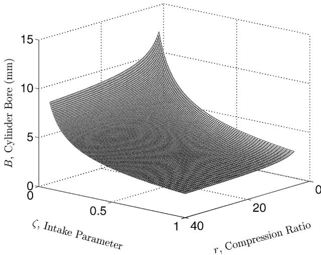
Fig. 4. The cylinder bore dependence upon the compression ratio and intake conditions for a non-supercharged 10 W engine.  $\zeta = 1.0$  corresponds to  $P_i = 1$  atm,  $T_i = 300$  K, and  $\Phi = 1.0$ .
