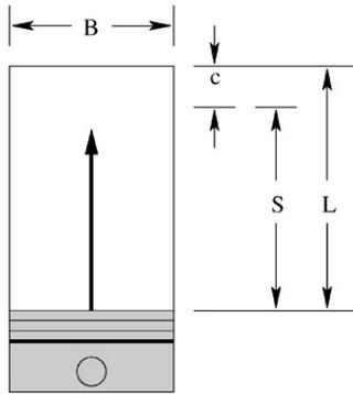
Fig. 2. Single cylinder engine geometry assumed in the performance analysis.
