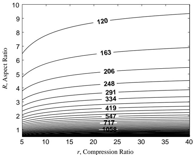
Fig. 7. Engine speed,  $N$  (Hz) required to deliver 10 W when operating with a mixture of propane and air,  $\Phi = 0.5$ ,  $T_i = 500$  K and  $P_i = 1$  atm ( $\zeta = 0.3$ ).
