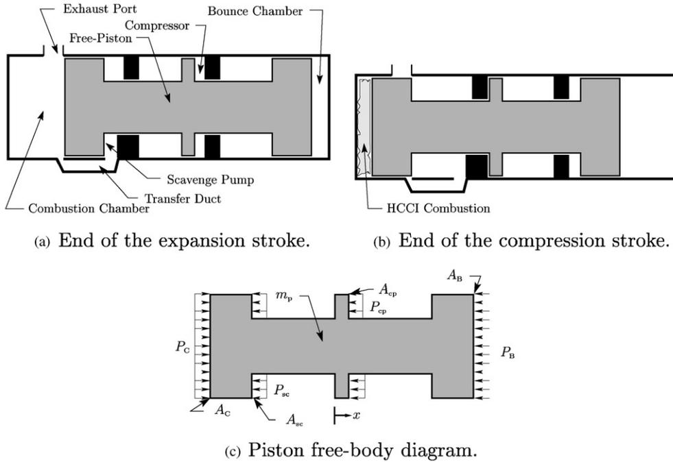
Fig. 1. Miniature free-piston engine concept (intake, compressed air outlet, and counter balance mechanism omitted). (a) End of the expansion stroke; (b) end of the compression stroke; (c) piston free-body diagram.
