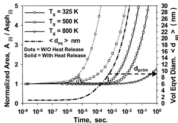
FIG. 7. Variation of silicon normalized area and mean volume equivalent diameter with residence time for various background gas temperatures,  $T_g$ ,  $P_g = 100$  Pa, and particle volume loading,  $\phi = 10^{-6}$  ( $A_{(i)}$ : particle area and  $A_{sph(i)}$ : equivalent spherical area of the corresponding particle).
