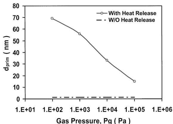
FIG. 14. The effect of background gas pressures ( $P_g$ ) on primary particle sizes ( $d_{prim}$ ) for titania nanoparticle coalescence at  $T_g = 1600$  K, and particle volume loading,  $\phi = 10^{-3}$ . Primary particle size without the heat release effect has also been indicated.
