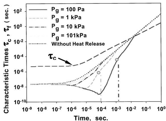
FIG. 8. Variation of characteristic coalescence/fusion ( $\tau_f$ ) and characteristic collision ( $\tau_c$ ) times with residence time for various background gas pressures,  $P_g$ ,  $T_g = 500$  K and particle volume loading,  $\phi = 10^{-6}$ . A gray point marks the gradient change for  $\tau_f$  corresponding to the point where  $A/A_{\text{sph}} \geq 1$ . Results are for silicon.
