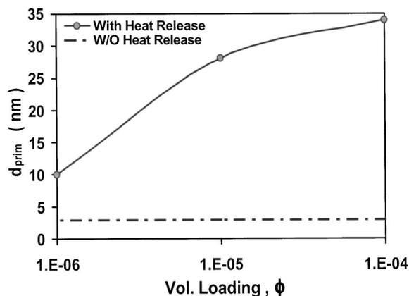
FIG. 16. The effect of particle volume loading ( $\phi = 10^{-4}, 10^{-5}, 10^{-6}$ ) on the prediction of primary particle sizes ( $d_{prim}$ ) for silicon nanoparticle coalescence  $T_g = 500$  K and gas pressure,  $P_g = 100$  Pa. Primary particle size predicted without heat release effect has also been indicated.
