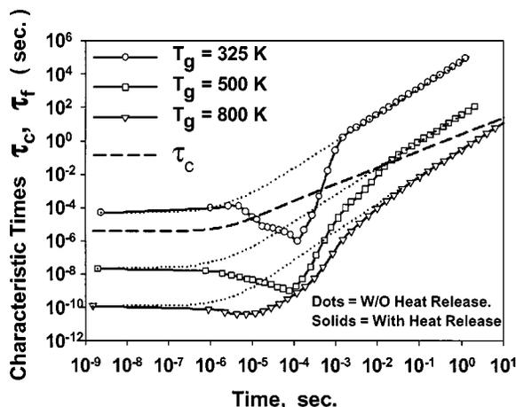
FIG. 5. Variation of characteristic fusion ( $\tau_f$ ) and collision ( $\tau_c$ ) times with residence time for various background gas temperatures for silicon (gas pressure,  $P_g = 100$  Pa and volume loading,  $\phi = 10^{-6}$ ).
