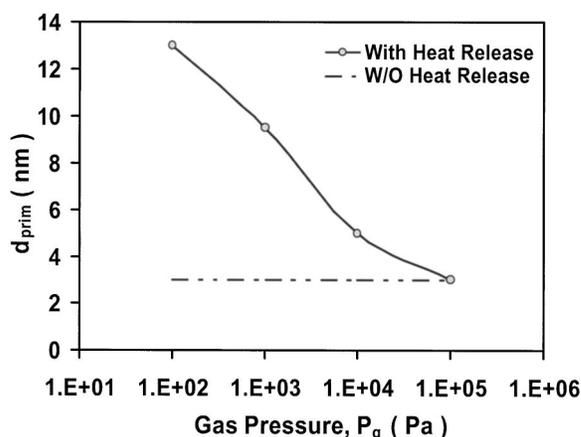
FIG. 10. The effect of background gas pressures ( $P_g$ ) on primary particle size ( $d_{\text{prim}}$ ) for silicon nanoparticles at constant gas temperature,  $T_g = 500$  K and particle volume loading,  $\phi = 10^{-6}$ . The primary particle size predicted without a heat release effect has also been indicated.
