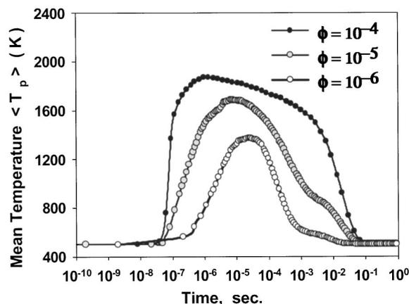
FIG. 15. The effect of different particle volume loading ( $\phi = 10^{-4}, 10^{-5}, 10^{-6}$ ) on the temporal variation of the mean particle temperature ( $\langle T_p \rangle$ ) at constant gas temperature  $T_g = 500$  K and gas pressure  $P_g = 100$  Pa for silicon nanoparticle coalescence.
