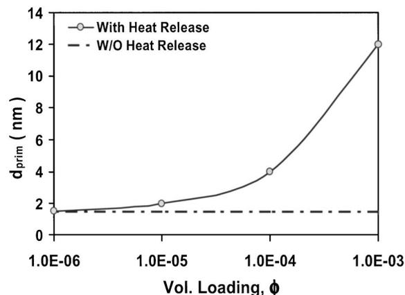
FIG. 18. The effect of particle volume loading ( $\phi = 10^{-3}, 10^{-4}, 10^{-5}, 10^{-6}$ ) on the prediction of primary particle sizes ( $d_{\text{prim}}$ ) for titania nanoparticle coalescence,  $T_g = 1600$  K, and gas pressure,  $P_g = 101$  kPa (1 atm). A primary particle size without heat release effect has also been indicated.
