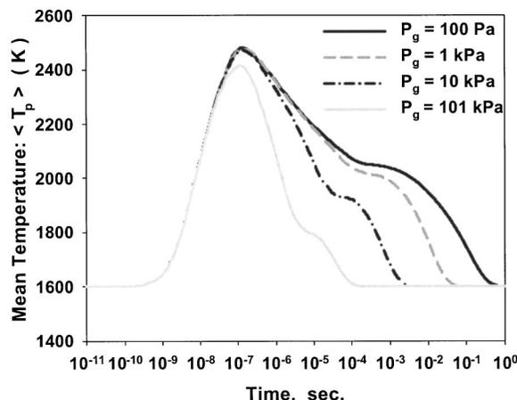
FIG. 13. The variation of the mean particle temperature ( $\langle T_p \rangle$ ) with residence time for various background gas pressures,  $P_g$ ,  $T_g = 1600$  K, and particle volume loading,  $\phi = 10^{-3}$  for titania nanoparticle coalescence.
