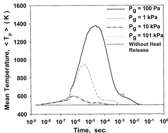
FIG. 9. The variation of mean silicon particle temperature ( $\langle T_p \rangle$ ) with residence time for various background gas pressures,  $P_g$ ,  $T_g = 500$  K, and particle volume loading,  $\phi = 10^{-6}$ . A gray point marks the gradient change for  $\tau_f$  corresponding to the point where  $A_{(t)}/A_{\text{sph}(t)} \geq 1$ .
