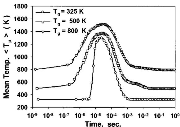
FIG. 6. Variation of mean silicon particle temperature ( $\langle T_p \rangle$ ) with residence time for various background gas temperatures,  $T_g$ , at constant gas pressure,  $P_g = 100$  Pa, and particle volume loading,  $\phi = 10^{-6}$ .
