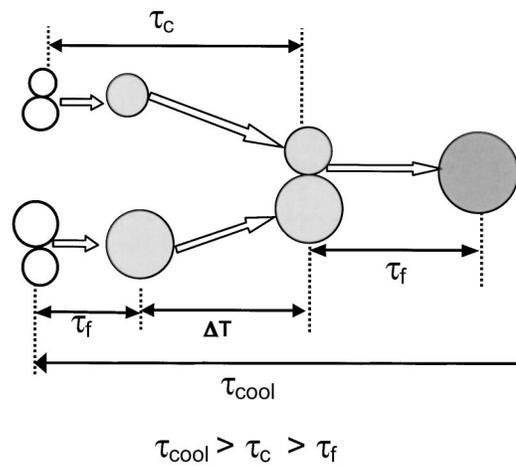
FIG. 2. The schematic diagram indicating the various time scales; mean interevent time ( $\Delta T$ ), characteristic coalescence/fusion ( $\tau_f$ ), characteristic collision ( $\tau_c$ ), and the mean cooling time for particles ( $\tau_{cool}$ ).
