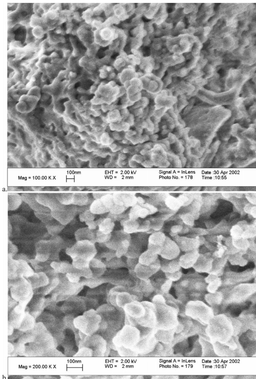
**Figure 4.** SEM images of the Al/C<sub>13</sub>F<sub>27</sub>COOH composite at (a) 100K and (b) 200K magnification.
