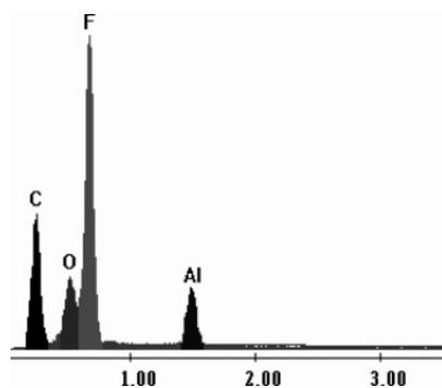
**Figure 6.** EDAX spectrum of the Al/C<sub>8</sub>F<sub>17</sub>COOH composite showing relative intensities of X-ray emission peaks assigned to C, O, F, and Al.
