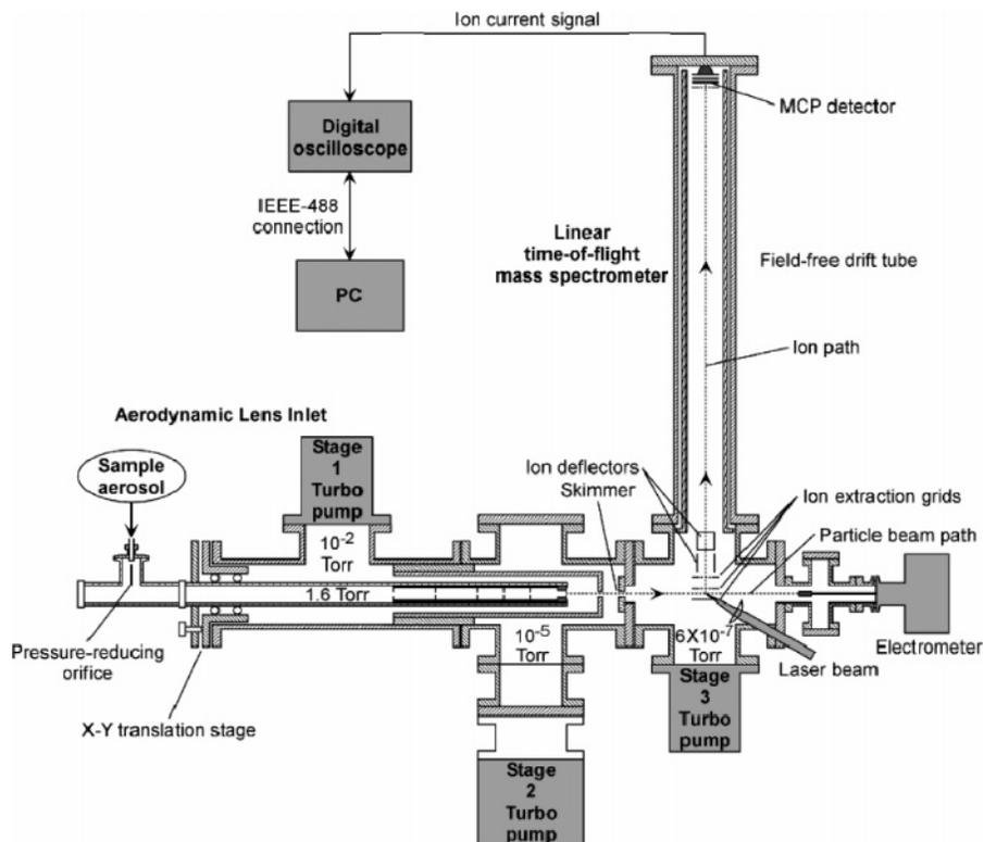
**Figure 1.** Schematic of single-particle mass spectrometer (SPMS).
