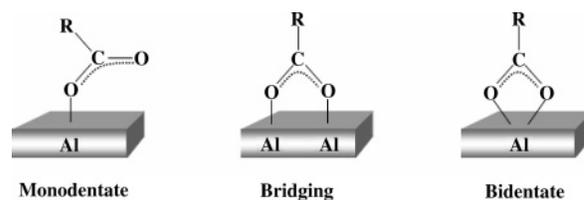
**Figure 8.** Three proposed structures for carboxylate binding to Al surface. In the monodentate geometry only one oxygen atom is bonded to the aluminum surface. For the bidentate coordination, the oxygen atoms are both bonded to the same aluminum atom. In the bridge-bonded configuration, the oxygen atoms are identical but on different aluminum atoms.
