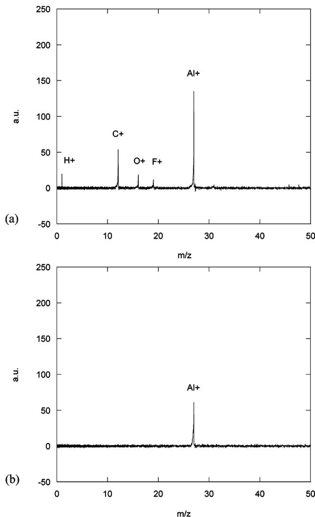
**Figure 11.** Typical mass spectra for (a) Al/C<sub>13</sub>F<sub>27</sub>COOH particles and (b) pure aluminum nanoparticles measured with SPMS at 25 °C.
