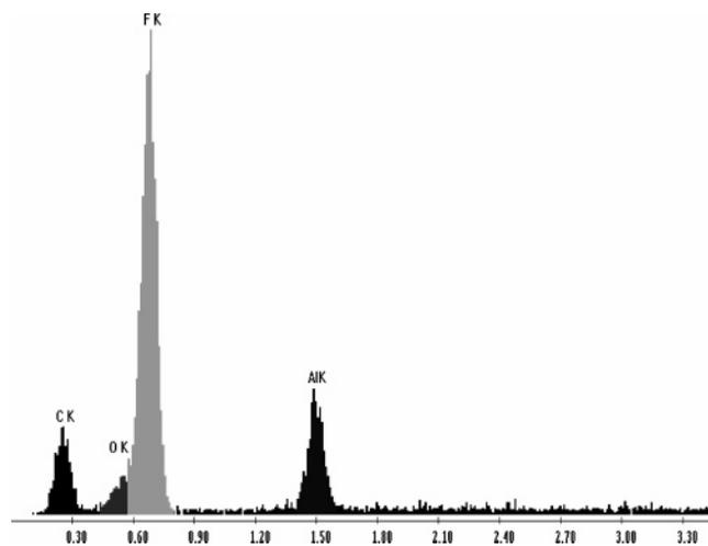
**Figure 5.** EDAX spectrum of the Al/C<sub>13</sub>F<sub>27</sub>COOH composite showing relative intensities of X-ray emission peaks assigned to C, O, F, and Al.
