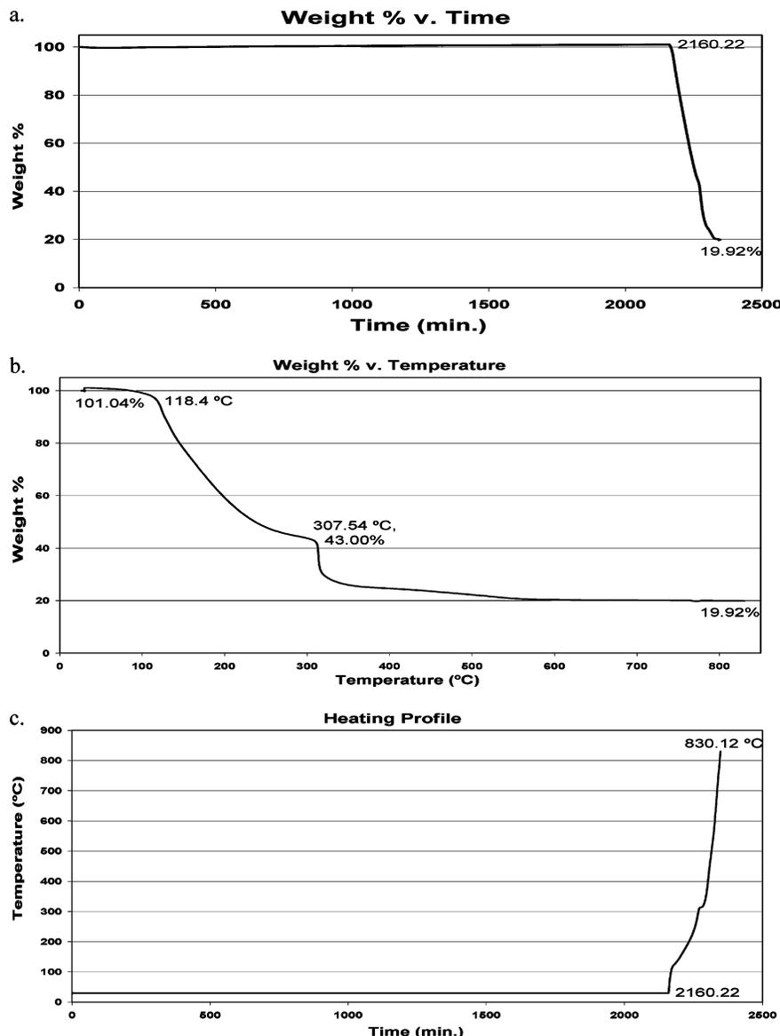
**Figure 3.** Thermogravimetric analysis of the Al/C<sub>13</sub>F<sub>27</sub>COOH composite showing (a) the stability of the material in air, weight vs time; (b) thermal decomposition/combustion in air, weight vs time; and (c) the heating profile of the experiment, temperature vs time.
