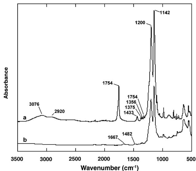
**Figure 7.** ATR-FTIR spectrum of the free perfluorotetradecanoic (C<sub>13</sub>F<sub>27</sub>COOH) acid (a) and the Al/C<sub>13</sub>F<sub>27</sub>COOH composite material (b).
