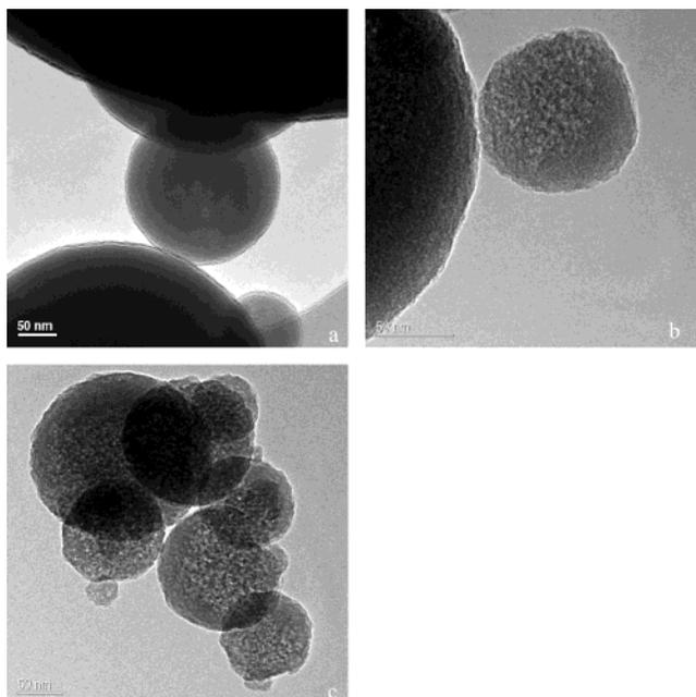
**Figure 3.** TEM images of silica particles: (a) TEOS/EtOH/H<sub>2</sub>O/HCl/NaCl = 1:22:60:30:0 ( $t_H = 20$  h), (b) TEOS/EtOH/H<sub>2</sub>O/HCl/NaCl = 1:22:60:30:2 ( $t_H = 20$  h), and (c) TEOS/EtOH/H<sub>2</sub>O/HCl/NaCl = 1:22:60:30:2 ( $t_H = 50$  h).
