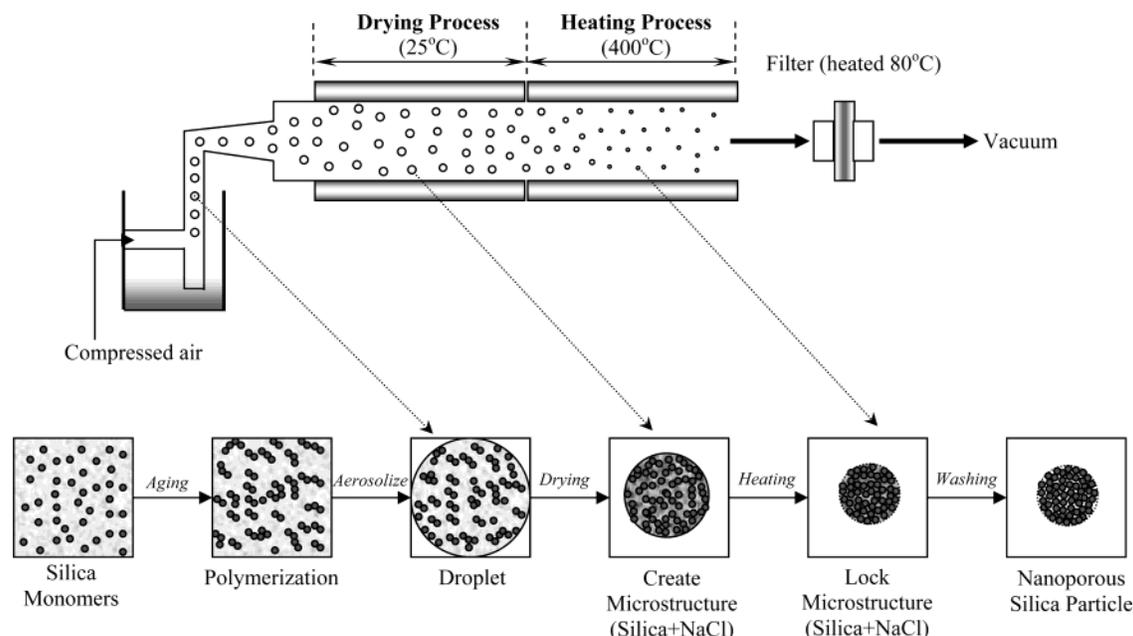
**Figure 1.** The schematic of the experimental setup and an illustration of the possible pathway of nanoporous silica particle formation.
