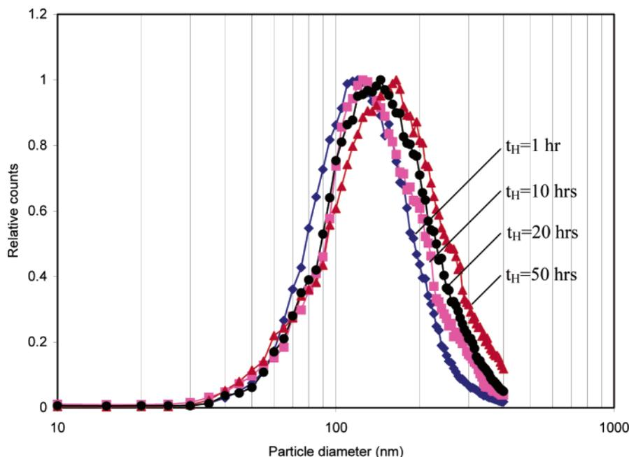
**Figure 2.** Particle size distribution for various aging times of the precursor solution (TEOS/EtOH/H<sub>2</sub>O/HCl/NaCl = 1:22:60:30:2).
