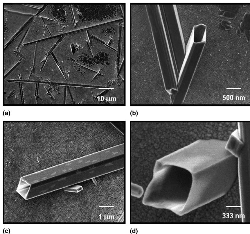
FIG. 2. Micrographs of hollow microducts grown from the tungsten film, at different magnifications.
