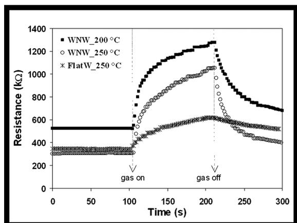
FIG. 7. Gas-sensor response curves from an annealed nanowire-coated surface and an annealed flat tungsten thin film surface, both exposed to 20 ppm of test gas  $\text{NO}_2/\text{NO}$ .
