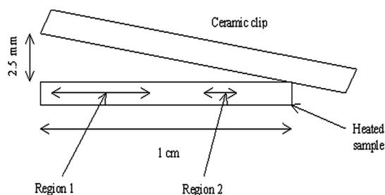
FIG. 5. Schematic of sample-clip assembly; Region 1 is covered with nanowires, while Region 2 contains microducts in addition to crystallite structures.
