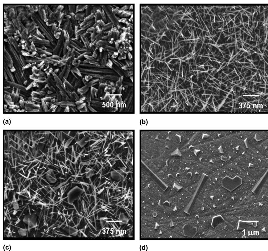
FIG. 1. Micrographs of tungsten film surface: (a) heated in the absence of  $\text{H}_2$ ; (b) nanowires; (c) nanowires and crystallite structures; (d) crystallite structures and solid square nanorods.
