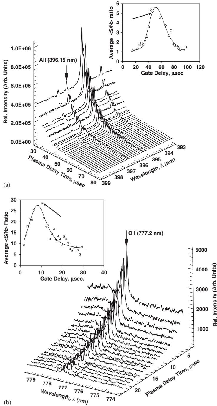
Fig. 6. Typical time-resolved atomic emission spectra of (a) Al I (396.15 nm) and (b) O I (777.2 nm) collected from laser-induced breakdown of  $Al_2O_3$  aerosol. Gate delays range (a) 30–80  $\mu$ s and (b) 5–25  $\mu$ s. The inset figure shows the variation of average signal/noise ratio ( $\langle S/N \rangle$ ) with gate delay times with the arrow indicating the optimal gate delay time chosen. The solid line indicates the best fit to the experimental data.
