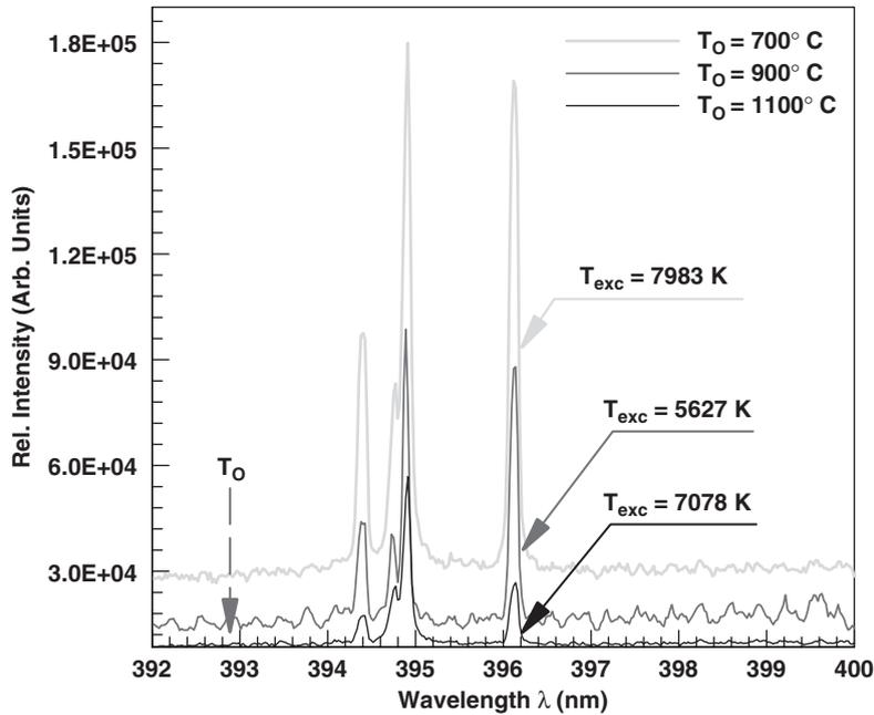
Fig. 9. Relative emission intensities of Al I (396.15 nm) signals collected at a delay time of 46.7  $\mu$ s for Al nanoparticles oxidized at three different oven temperatures ( $T_O = 700, 900, 1100^\circ\text{C}$ ). The respective plasma temperatures for each of the samples have been indicated as  $T_{\text{exc}}$  (K). All spectra shown have been shifted along the y-scale for ease of visualization.
