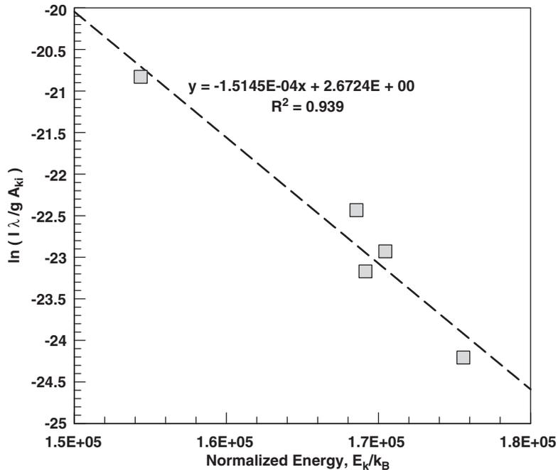
Fig. 12. Typical linear Boltzmann plot for five Ar I transition lines used to calculate plasma temperature,  $T_{\text{exc}}$ , for estimating aluminum number densities in  $\text{Al}_2\text{O}_3$  aerosol samples ( $T_{\text{exc}} = 1/\text{slope} = 6603 \text{ K}$  at delay time =  $46.7 \mu\text{s}$ ). Plot also shows linear fit to the data with a regression coefficient of  $R^2 \sim 0.939$ .
