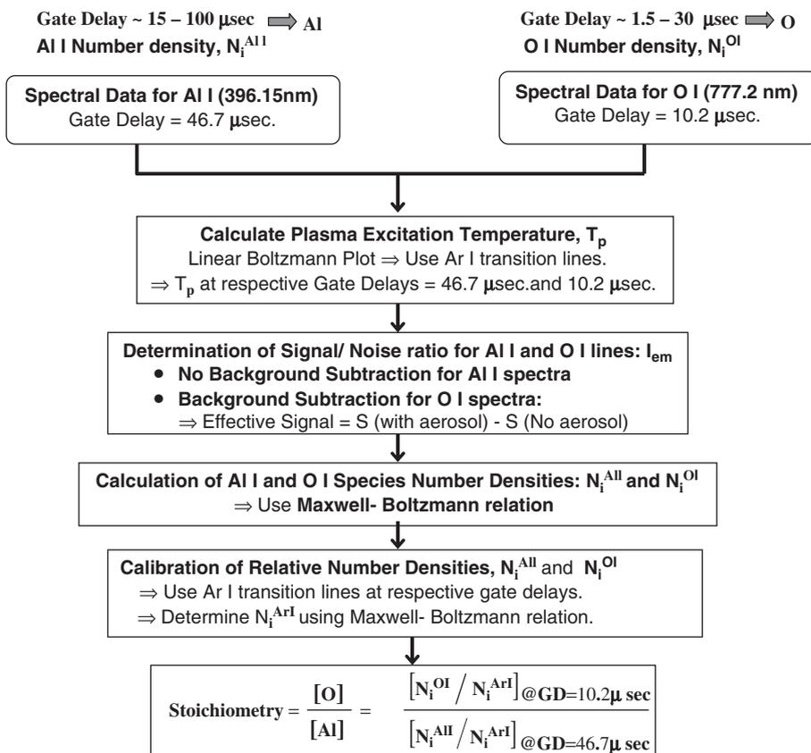
Fig. 5. Flow chart showing the methodology for quantitative spectral data analysis.
