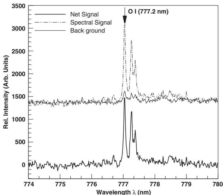
Fig. 7. Representative atomic transition line of O I (777.2 nm) collected for  $\text{Al}_2\text{O}_3$  aerosols at delay time = 10.2  $\mu\text{s}$  and gate width = 3.5  $\mu\text{s}$ . The “Net Signal” spectrum indicates the background subtracted spectral signal intensity.
