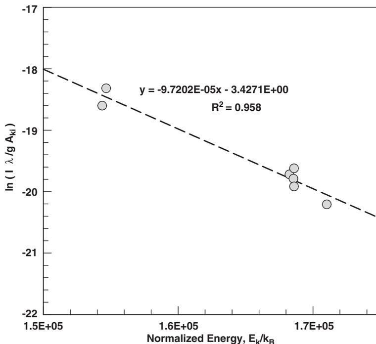
Fig. 11. Typical linear Boltzmann plot for seven Ar I transition lines used to calculate plasma temperature,  $T_{\text{exc}}$ , for estimating oxygen number densities in  $\text{Al}_2\text{O}_3$  aerosol samples ( $T_{\text{exc}} = 1/\text{slope} = 10,288 \text{ K}$  at delay time =  $10.2 \mu\text{s}$ ). Plot also shows linear fit to the data with a regression coefficient of  $R^2 \sim 0.958$ .
