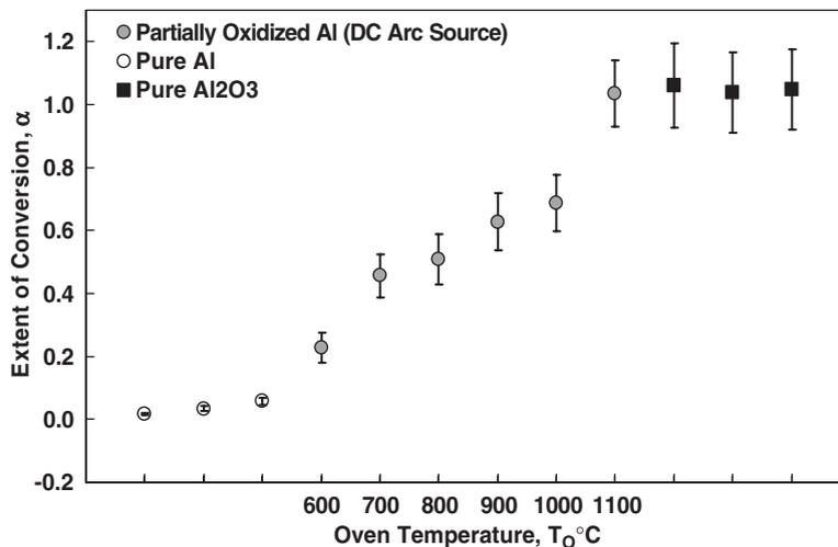
Fig. 13. Extent of oxidation in air,  $\alpha$ , of Al nanoparticles as a function of oxidation temperature. The oven temperature scale only extends between 600 and 1100 °C. Data points below 600 °C and above 1100 °C are for pure Al and Al<sub>2</sub>O<sub>3</sub> aerosols used as reference points.
