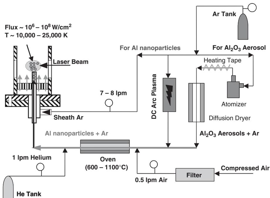
Fig. 1(b). Schematic for aerosol supply system.
