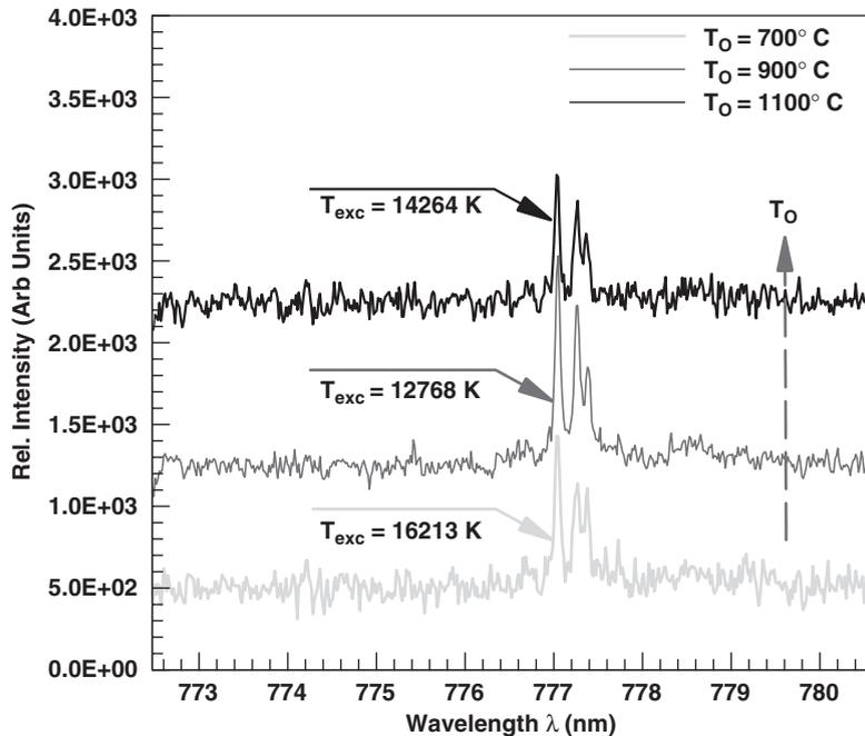
Fig. 10. Relative intensities of background subtracted net emission signals of O I (777.2 nm) at a delay time of 10.2  $\mu$ s for Al nanoparticles samples oxidized at three different oven temperatures ( $T_O = 700, 900, 1100^\circ\text{C}$ ). The respective plasma temperatures calculated at 10.2  $\mu$ s delay time have been indicated as  $T_{\text{exc}}$  (K). All spectra shown have been shifted along the y-scale for ease of visualization.
