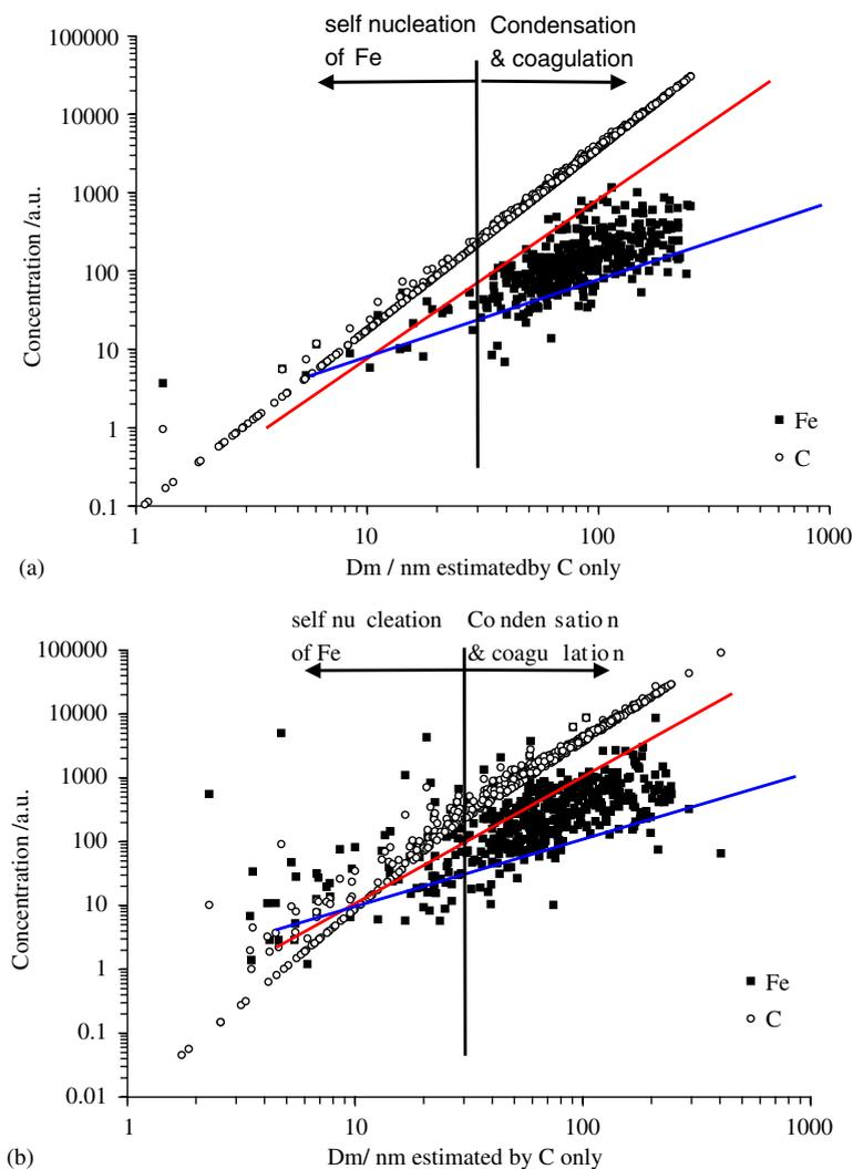
Fig. 12. Size dependence of iron and carbon fractions in diesel exhaust particles for the case of low-Fe doping: (a) 0 W load, and (b) 6 kW load. (Note that upper line shows  $D_{m,c}^2$  while lower line shows  $D_{m,c}^1$ .)
