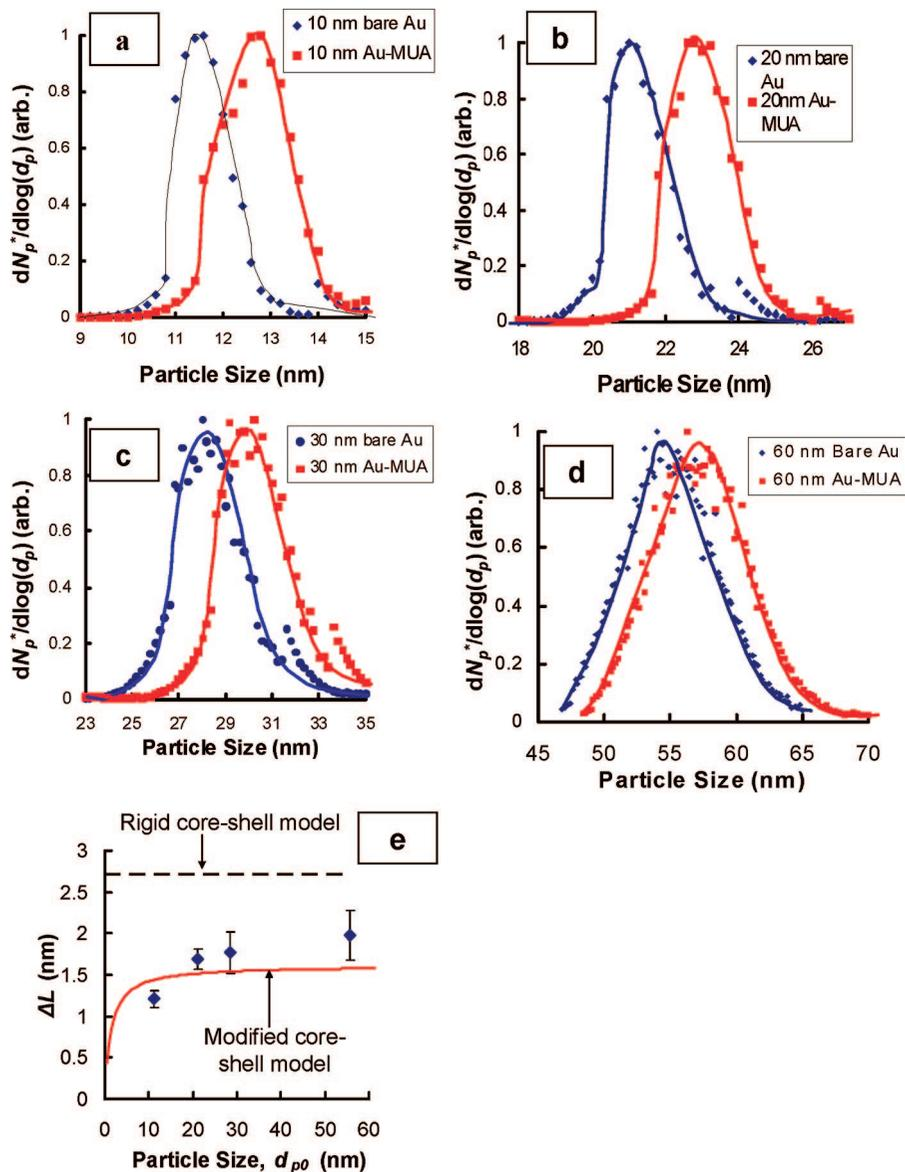
**Figure 4.** Particle size distributions of bare vs MUA-coated Au-NP for (a) 10 nm particles (b) 20 nm (c) 30 nm, and (d) 60 nm. (e) Comparison of predicted  $\Delta L$  from experiment (diamonds) with theory ( $\Delta L_1$  as dashed line and  $\Delta L_2$  as solid line).
