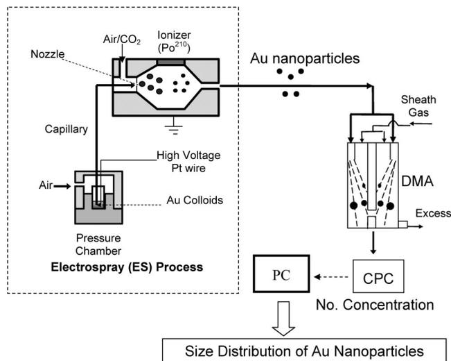
**Figure 1.** Schematic of experimental system, including differential mobility analyzer (DMA) and condensation particle counter (CPC).
