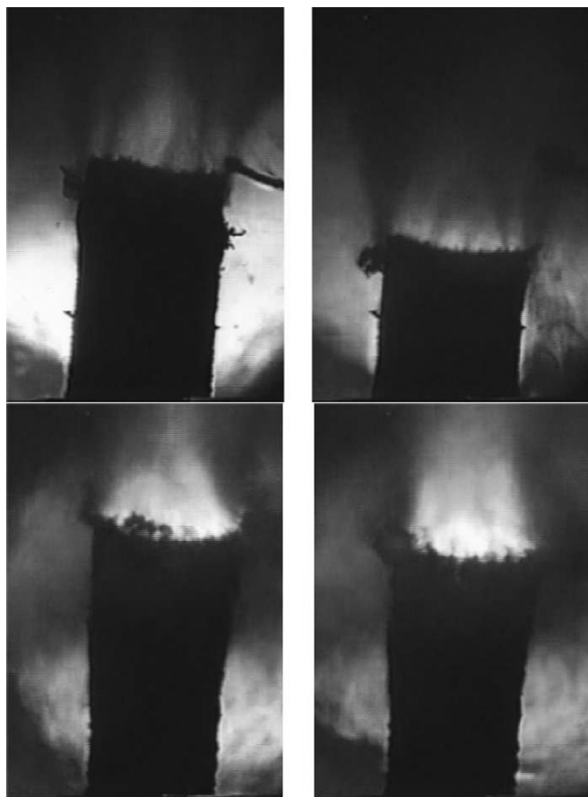
Figure 4. Captured video images of baseline (top) and mesoparticle (bottom) propellant burning in strand burner at 4.25 MPa. Note luminosity increase in mesoparticle based propellant.
