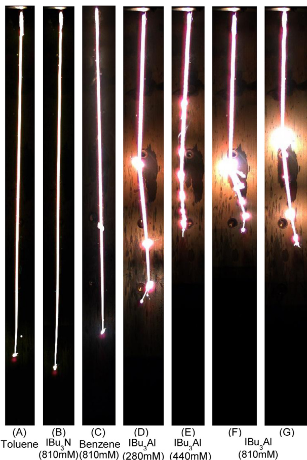
Fig. 1. Representative time-lapse images of free-falling droplets combusting with and without various additives. (A) Pure toluene, (B) 810 mM IBu 3 N in toluene, (C) 810 mM benzene in toluene, (D–E) 280 mM and 440 mM IBu 3 Al in toluene, (F–G) Two types of disruptions from 810 mM IBu 3 Al in toluene. The mid-height emission expansion in (C) is an artifact caused by reflection off a spot of residue on the experiment cover glass and is not a disruption.
